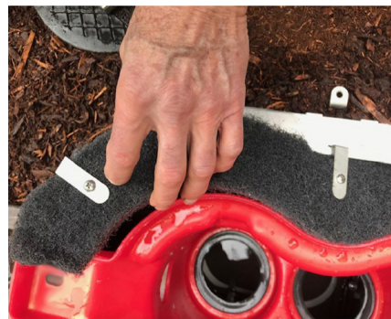
STEP 5: Remove poly-mat, overflow flush tubes and filter baskets.
