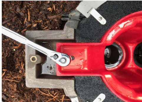
STEP 4: Remove the bolt at the back of the filter carriage.
